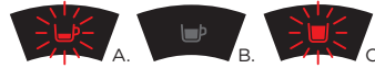
Fig. 20: Luminous alert that there is a lack of water in the water tank.
